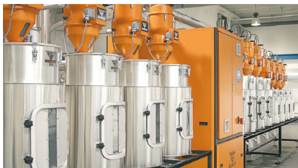
CKT 500 granule dryer with 12 drying containers
