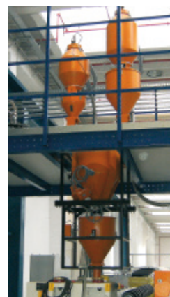
GRAVIKO GK 1000 with Loss-in-Weight control unit in use
